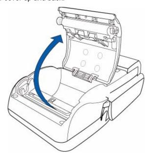
Figure 9 Opening the Printer Cover
